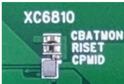
WLP-12-01 (1.17 x 1.57 x 0.33 mm) Ultra-small package and a few external components provide a space-saving, low-profile solution.
